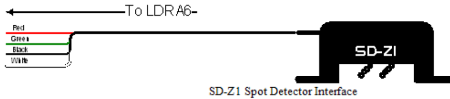
Figure 3.2 SD-Z1 Spot Detector Connection
