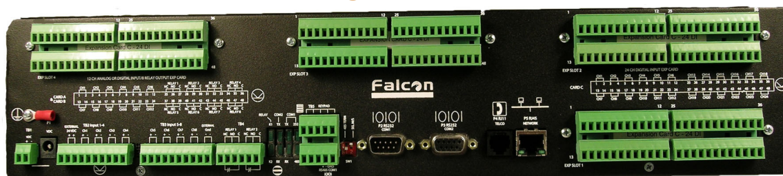
Figure 1.2 FMS Terminal Block Designations
